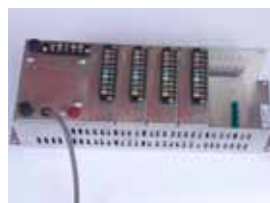
CRL 103 Power Unit Mainframe + four CRL 104 Power Unit Channels
